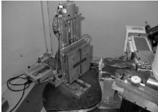
Fig. 4: Automated x-ray diffraction residual stress measurement apparatus with FSW mounted for residual stress mapping.
