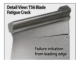
Low Plasticity Burnishing (LPB®) mitigates pitting, diminishes foreign object damage (FOD), and improves damage tolerance and high cycle fatigue (HCF) while reducing the replacement costs of the 17-4 PH Stainless Steel 1st Stage Compressor Blade in the T56 Turboprop Engine.
