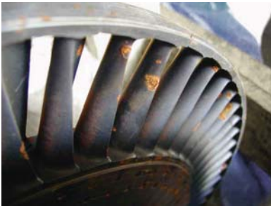
Corrosion Pitting in Steam Turbine Blades
